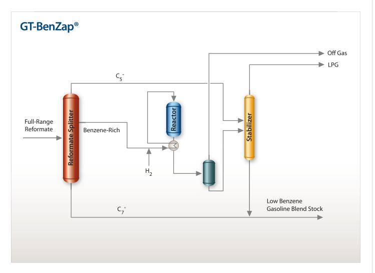
A narrow-cut C<sub>6</sub> fraction is first separated from the full-range reformate and then hydrogenerated to saturate benzene and contained olefins. The reactor effluent is sent to a stabilizer to remove light components. There is an option to process C<sub>5</sub> from the reformate splitter in the same stabilizer. The stabilizer bottom stream is combined with  $C_7^+$  from the splitter bottom and sent to the gasoline pool as low-benzene blend stock.
